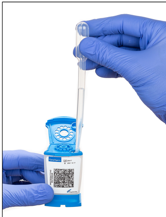
Figure 6. Dispensing Decontaminated Liquefied Sample into the Sample Chamber of the Cartridge
