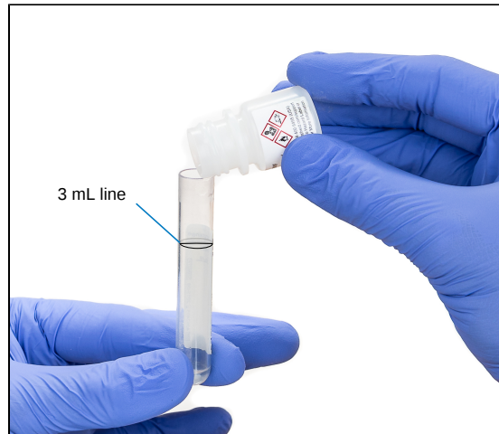
Figure 4. Example of 2:1 Dilution (2 mL SR:1 mL Sputum)
