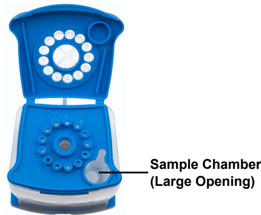
Figure 3. HIV-1 Qual XC Cartridge (Top View)
